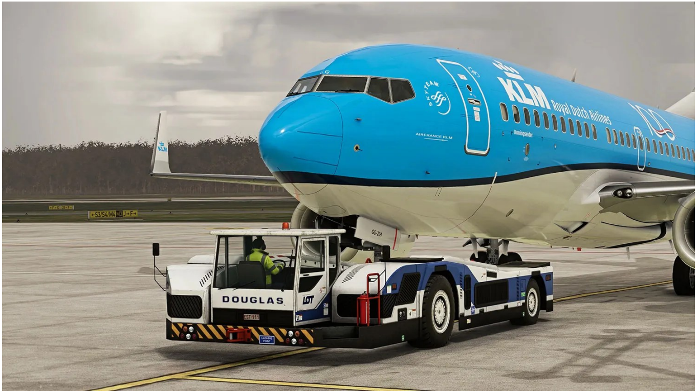
Pushback tractor at the nose of a Boeing 737
