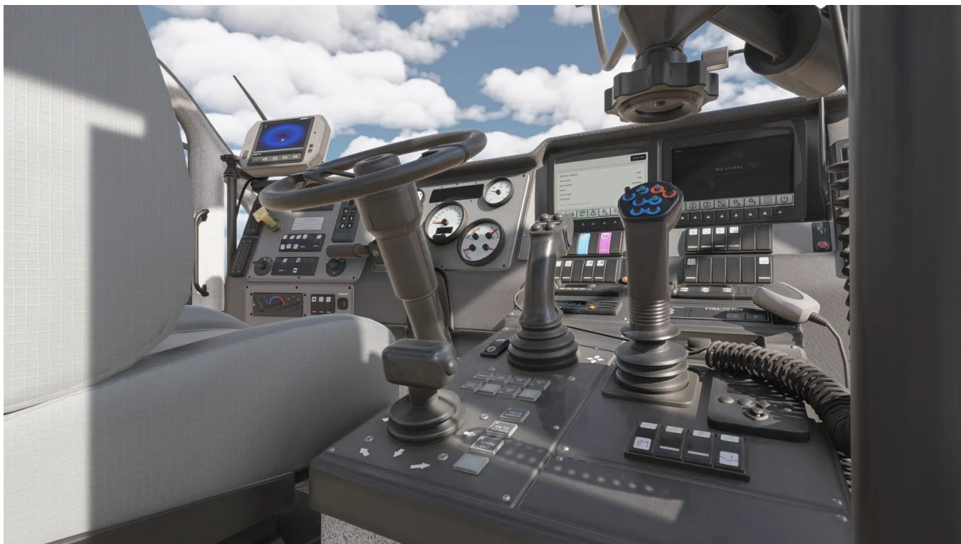
Modeled ARFF cabin with joysticks and displays
